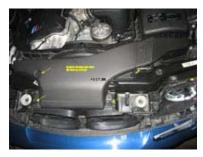
**2d) Remove the H7 bulb from (flasher) socket and peel the rubber boot back.** Surrounding the H7 bulb socket is a rubber boot. Peel back on the boot from the top to allow you to pass the Angel Eye wires through.
