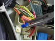
**4c)** Route the red trigger wire into the ECU box and connect the terminal end to the blue wire tap. I chose to lift one of the rubber grommets and lay the red trigger wire underneath. You can fish it through the grommet if you like for a more professional look.
