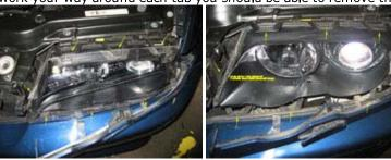
1e) Remove the OEM inner trim bezel. The bezel simply pulls straight out. No tools needed.
