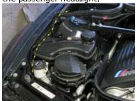
3d) Connect the passenger side angel eye harness to the relay harness.
